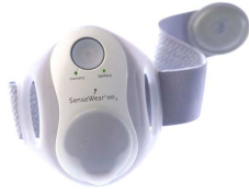
Fig. 5. Bodymedia Armband : hardware device to measure skin conductance.
