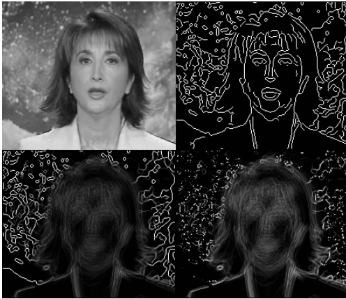
Fig. 2. Example of temporal X-ray transformation. From left to right, starting from the top: original frame, edge image, temporal X-ray image, filtered temporal X-ray image.
