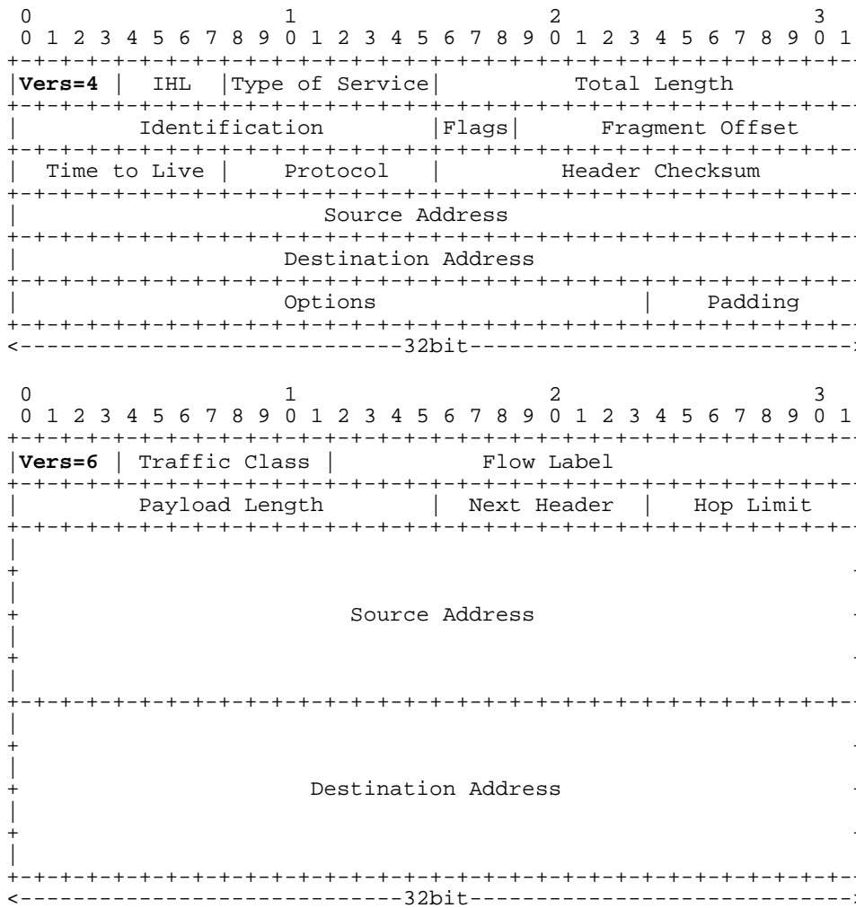
Figure 2: IPv4 Header (RFC791) & IPv6 Header (RFC1883 draft-ietf-ipngwg-ipv6-spec-v2-01)
