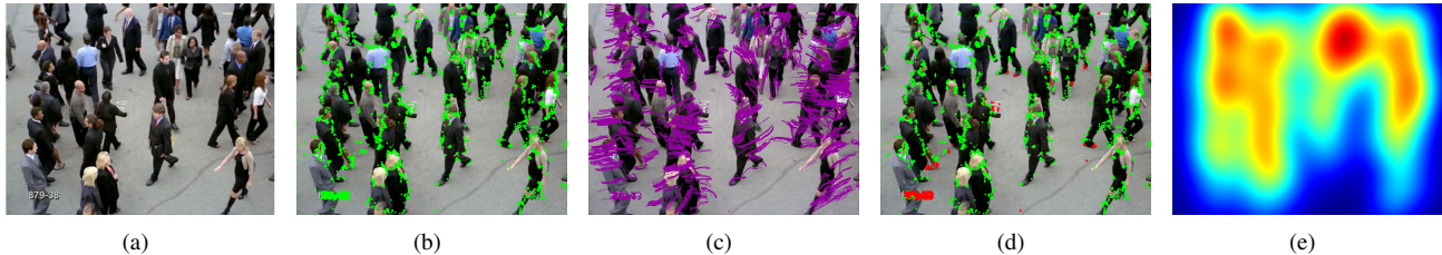
Figure 2. Illustration of the proposed crowd density map estimation using local features extraction: (a) Exemplary frame, (b) Local feature points (in this case by FAST algorithm), (c) Feature tracks, (d) Distinction of moving (green) and static (red) features - red features at the lower left corner are due to text overlay in the video, (e) Estimated crowd density map
