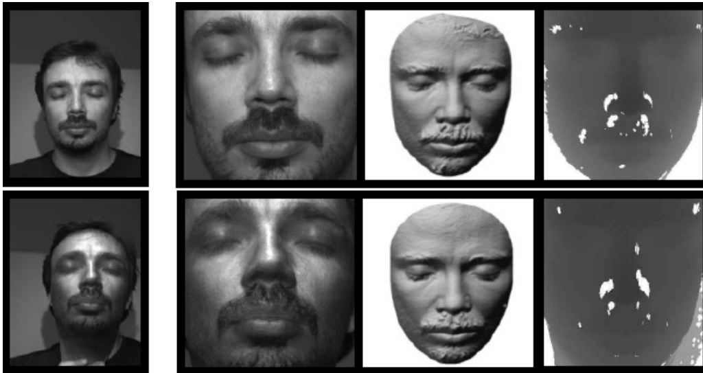
Figure 4.2: Example from the mask database which is created by MORPHO. From left to right (upper row) The real face, the cropped texture image, the 3D scan after preprocessing, the cropped depth map estimated from the raw 3D scan (lower row) same images for the corresponding mask attack.
