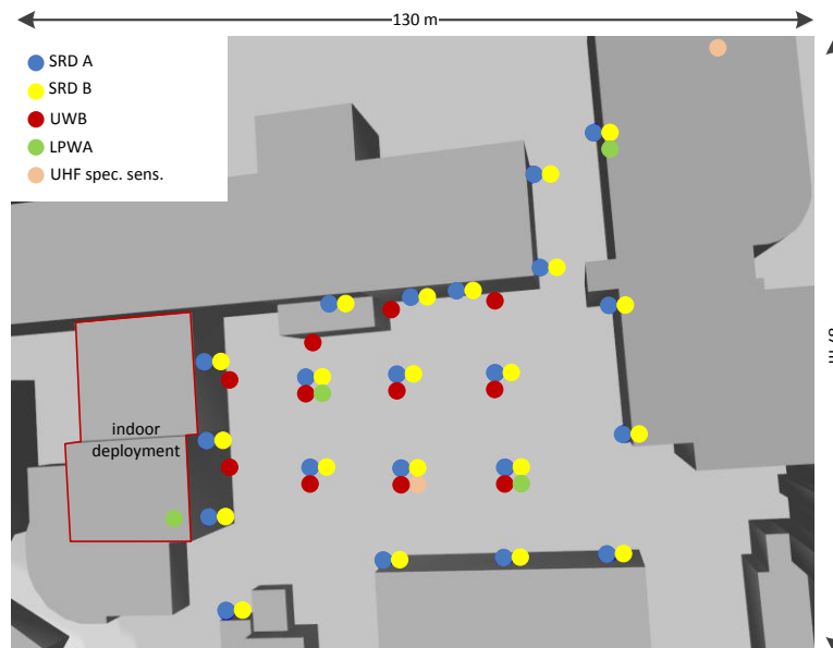
Fig. 4.6.2. Location of nodes in LOG-a-TEC testbed
