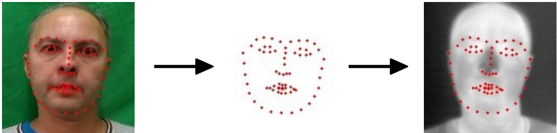
Figure 6.4: Ground truth facial landmark annotation of CSMAD data: facial landmarks are first detected on the visible images using DLIB [166] followed by manual verification and correction. The detected landmarks are simply used as ground truth for thermal images.
