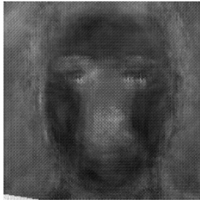
Figure 4: Pixel difference between original and synthesized depth maps: the lighter pixels around the nose and eyes areas show that it is more challenging to predict the correct depth value in those areas.
