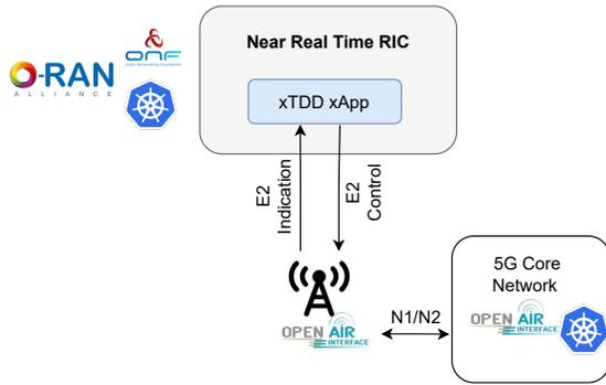
Figure 1: O-RAN aligned architecture of xTDD
