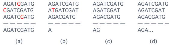
Figure 1: Example of consensus algorithm applied to a cluster of three strings in case of substitution errors only (a) and insertion/deletion errors (b)-(d).
