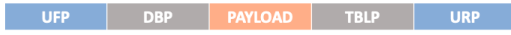
Figure 2: The oligo structure for object based abstraction. UFP/URP: universal forward/reverse primer, DBP: database primer, TBLP: table primer.
