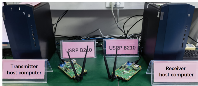
Fig. 1. An Explainable Semantics-based Image Semantic Communication (ES-ISC) System. This demo system runs on two host computers equipped with Ubuntu22.04 system and Nvidia RTX4060 graphics card. For on-site presentation, we need a desk to provide enough space for two host computers, two displays, keyboard and mouse, and also four three-legged sockets to power the computers and displays.
